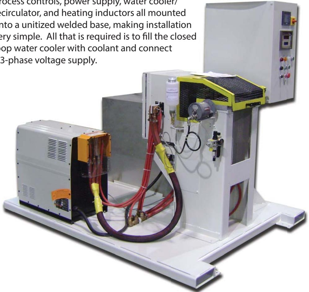
Ajax TOCCO Magnethermic's 35kW air cooled induction heating power supply is capable heating up to 115kg of steel per hour based on an 1100C temperature rise. Additional power supply offerings are available for varying production demands.
