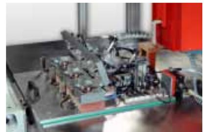
Interchangeable applications cassette with inert gas cover enclosures and induction coil assembly
