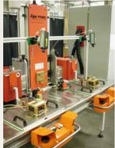
Integrated dual station system with optical pyrometer sensing
