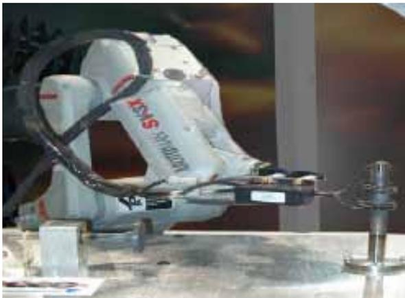
Adaptable robot configurations for "in-place" brazing
