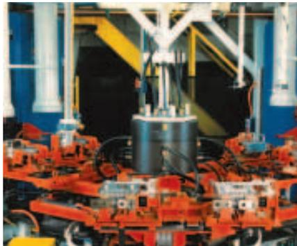
Six station compound motion for automated brazing of aluminum evaporator cores
