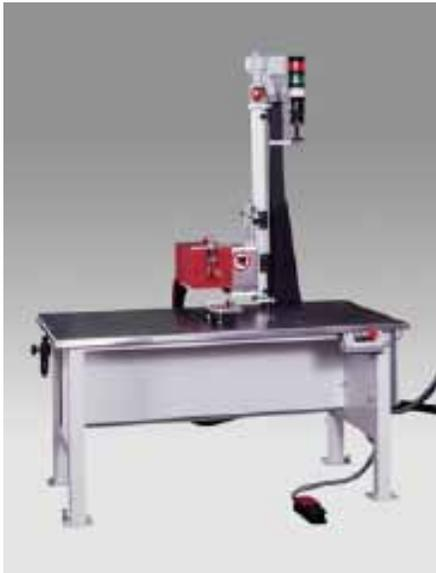
Universal single and dual station platforms are the foundations to integrate application specific features including shield gas controls, process tooling, coil assemblies, temperature sensing and process controls.
