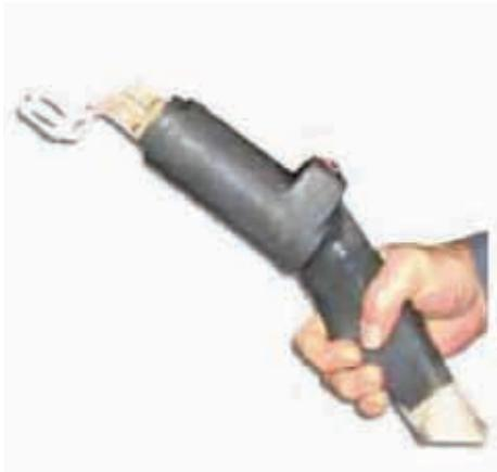
Hand-Held Transformer and Coil Assembly for remote heating locations. This assembly allows for freedom of movement of the coil into the braze area by an operator or attached to a robot end effector.
