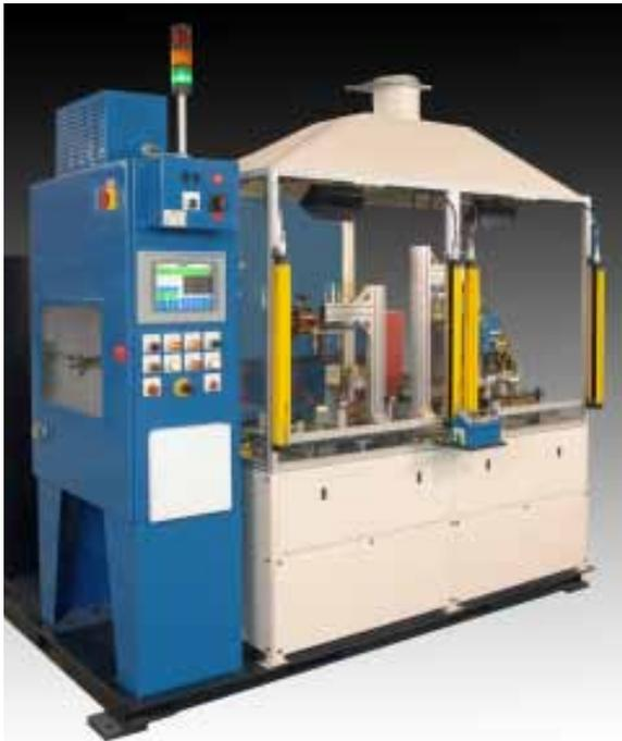
Unitized Dual Station Brazing System with integrated part program storage, illuminated working area and quick change tooling
