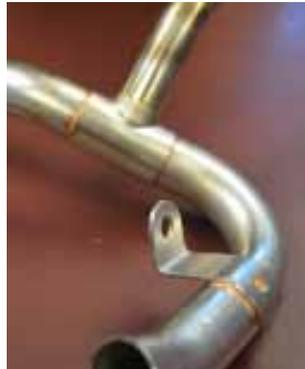
High temperature copper brazing of stainless to stainless tube assemblies in a shield gas fixture
