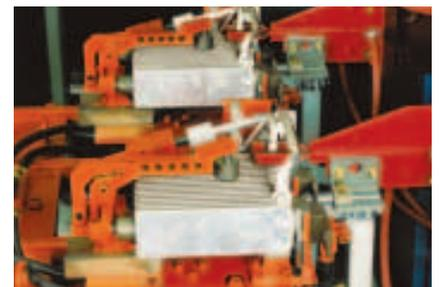
Aluminum brazing of tube-to-tube connections
