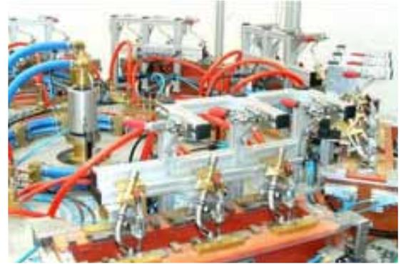
Independently controlled power supplies with braze tooling designed with chambers providing atmosphere cover of pure Nitrogen or Nitrogen/Hydrogen mixture
