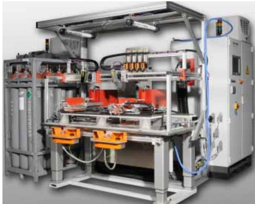
Dual station brazing cell with shield gas for fluxless brazing applications
