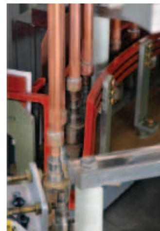
Rotary indexing soldering system featuring all stainless steel construction, alloy wire feeder and designed for high-volume production of non-ferrous tube and fitting assemblies.
