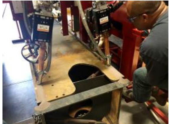
Each of the two inductors are positioned approximately 24 inches in front of two 1000-amp sub arc weld torches. The inductors and torches move in tandem. The weldment is simultaneously heated and welded as gantry traverses the length of the fillet.
