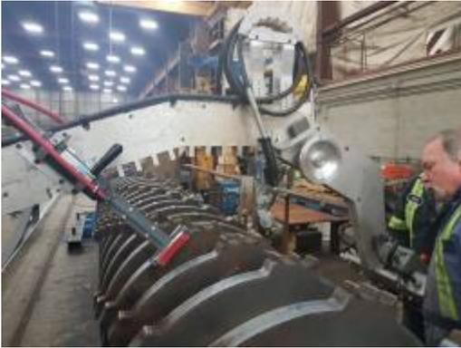
Ajax TOCCO Magnethermic recently supplied a forestry products manufacturer with a compact remote transformer and low profile heating inductor to be used for preheating prior to GMAW. These items were sold as a field install kit that are compatible with and utilize the customer's existing induction heating cables and accessories. The heating inductor floats above the weldment without making contact. Versatility and utilization of the 35 kW induction heater were immediately increased.
